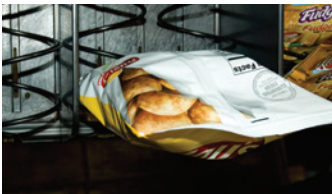
Incorrect Coil Sizing
